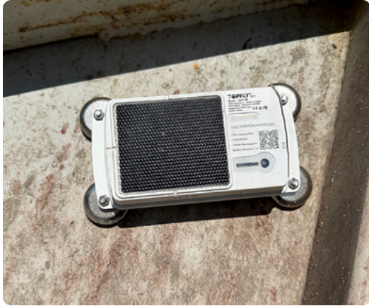
A solar tracker is attached to each Henriksen Washout bin to monitor location.
